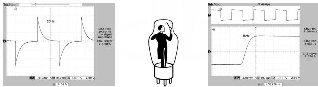
Input: 0.5mV<sub>RMS</sub>/10Ω + Cable 50pF Output: 47kΩ/100pF + Cable 50pF (no Impedance Correction, no Zobel-Network)
