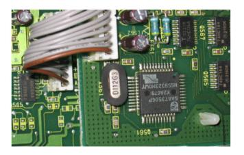
manual for CD-10, which I then studied intensively. I noticed that CD-10 houses a simple clock oscillator for the DAC as well as an Op-Amps at the audio output stage.
